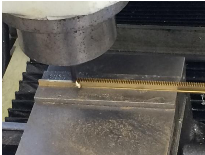
Figure 17: Tormach CNC-1100 from TechShop cutting the topmost edge of a brass leaf.
