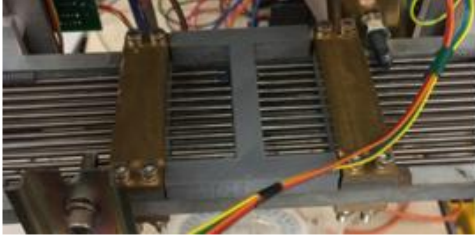
Figure 38: Initialized MLC. Leaves are manually set to touch the edges of a 1cm-thick plastic jig. The GUI then knows the absolute location of each leaf and can send relative commands.
