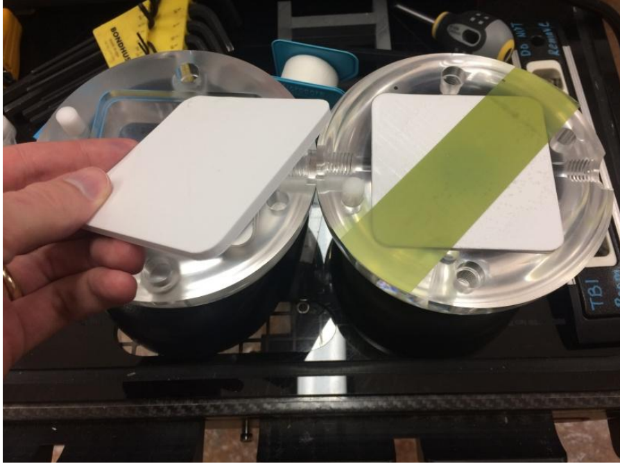
Figure 50: White inserts in the Lucy halves, with an example EBT3 strip as delivered.
