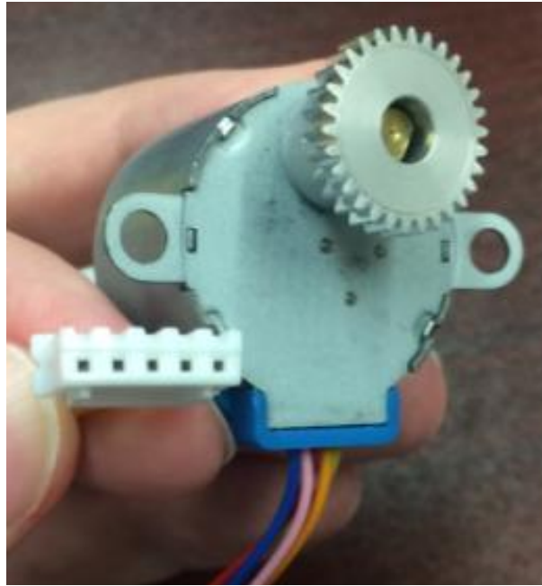
Figure 31: Stepper motor with gear attached, with five wires (bottom).
