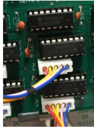
Figure 35: (Left) 74HC595 shift register schematic from Texas Instruments. (91) Output pins labeled QA-QH, 5V pin labeled VCC, clock pin labeled SRCLK, and latch pin labeled OE. (Right) A shift register (top black rectangle) feeding two Darlington arrays (bottom two black boxes) which feed stepper motor wires.
