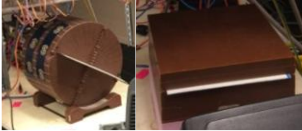
Figure 43: (Left) cheese phantom, loaded with an EDR2 envelope. (Right) solid water, each loaded with EDR2 film.
