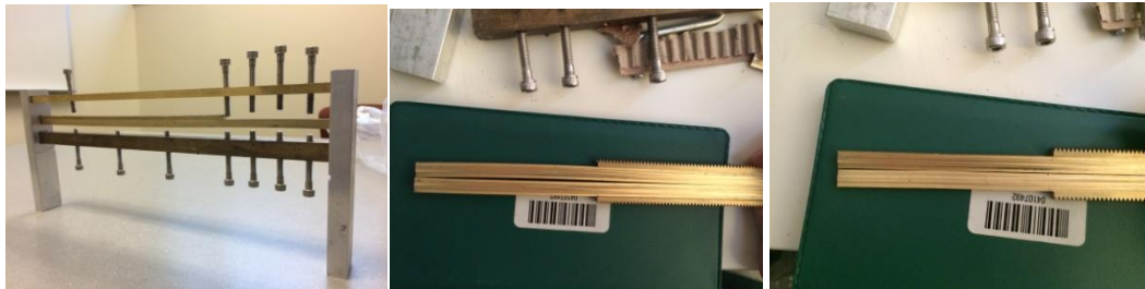
Figure 21: (Left) Straightening jig, (center) unstraightened leaves, (right) straightened leaves.
